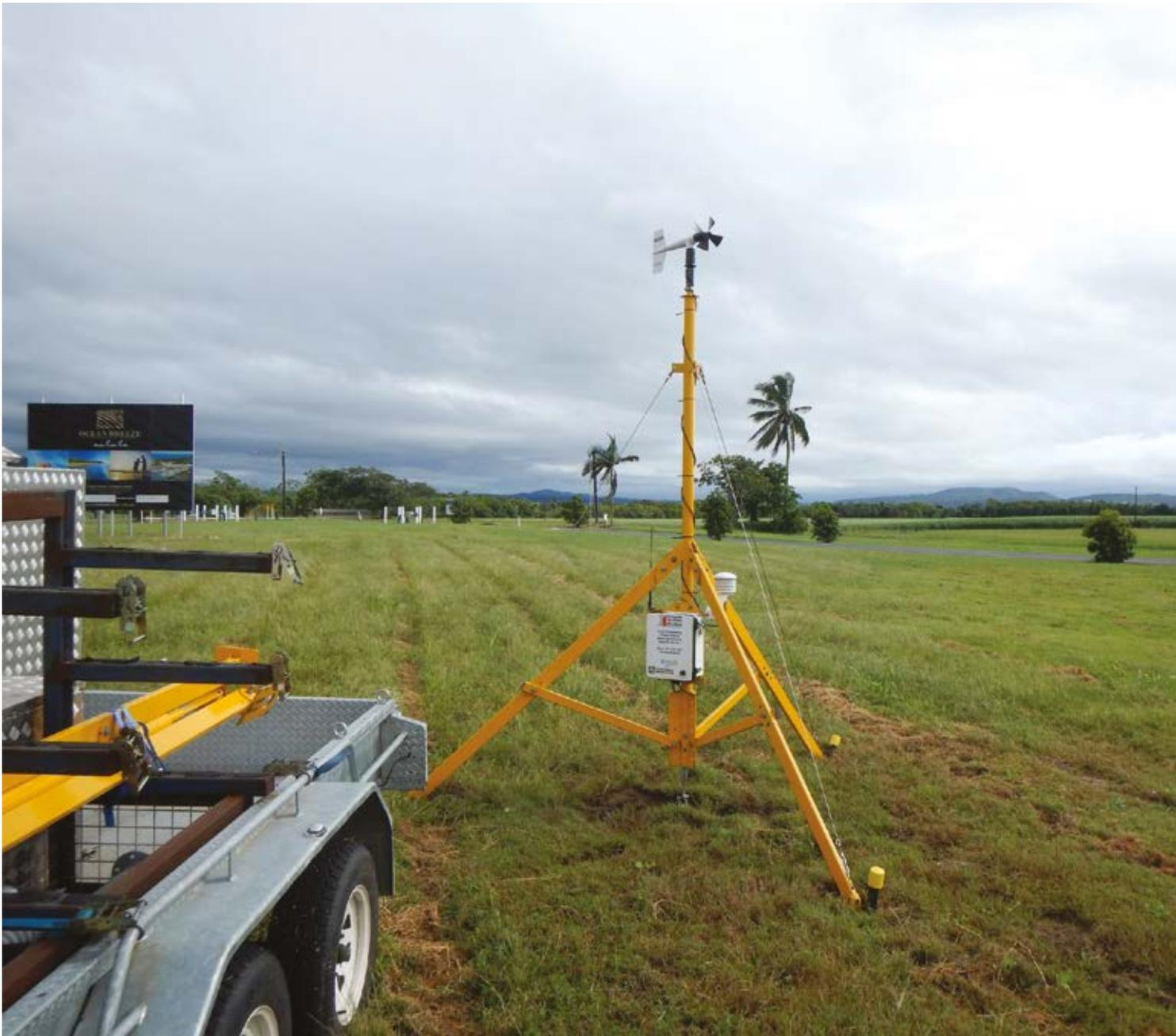
Cyclone Testing Station SWIRLNet anemometer, Cooktown: Portable wind station measuring wind speeds against Cyclone Ita 2014.
